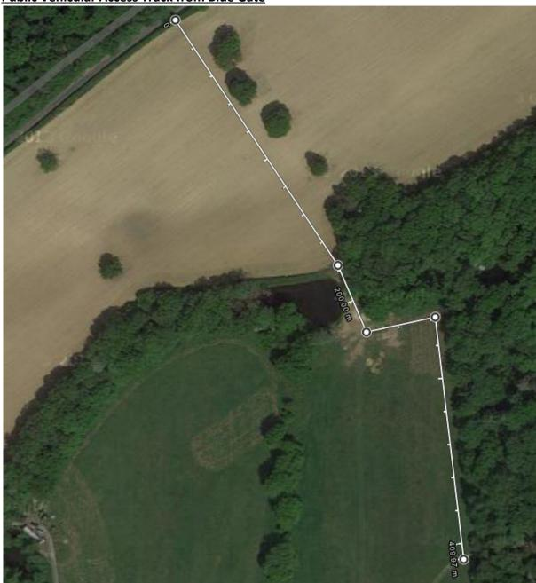
The Site has 400m of stacking space on hard standing, which equates to 120 cars in total, on average a B road sees 1 car every 10 seconds.
